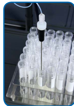
The SC-8 DX high-capacity oilFAST Autosampler holds as many as 720 8mL (90 position) sample vessels.
